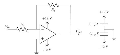
Figure 1: Inverting Amplifier Circuit
