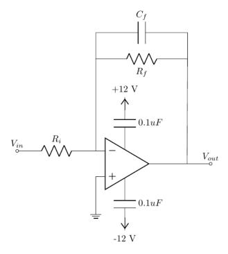
Figure 3: Active Low-Pass Filter Circuit
