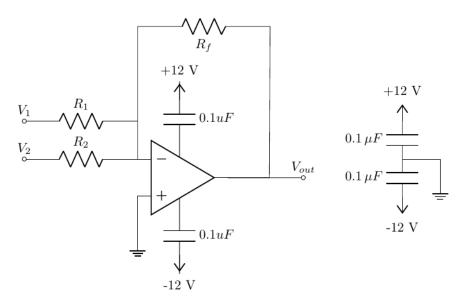
Figure 4: Summing Amplifier Circuit
