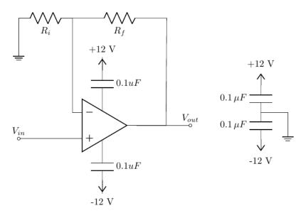
Figure 2: Non-Inverting Amplifier Circuit
